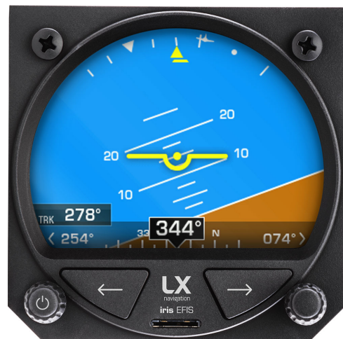
Figure 13. "Show airspeed" is disabled, "Show altitude" is disable and "Show direction" is set to "True Track"
