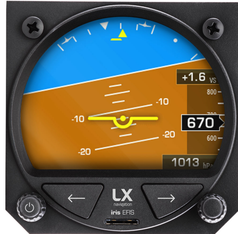
Figure 11. "Show airspeed" is disabled, "Show altitude" is disable and "Show direction" is set to "True Track"
