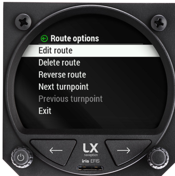
Figure 64. route options menu accessible - push left-hand push-rotary knob while at RTE page
