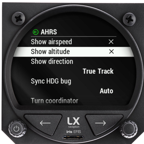
Figure 8. "Show airspeed", "Show altitude", "Show direction" options in setup page, graphic, AHRS menu
