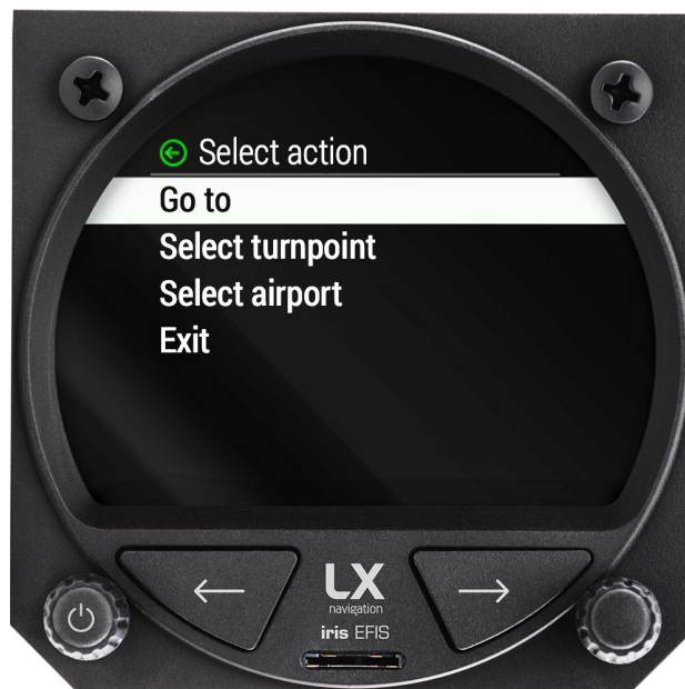
Figure 57. Selecting "T" (take-off) or "L" (landing) will take pilot to "Select action" menu
