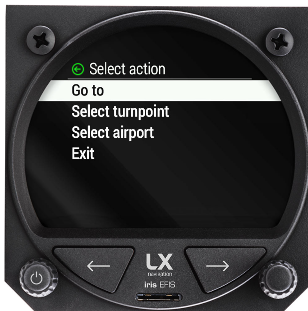
Figure 59. Selecting “T” (take-off) or “L” (landing) will take pilot to “Select action” menu
