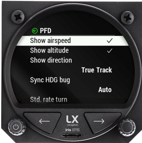
Figure 14. "Show airspeed", "Show altitude", "Show direction" options in setup page, "User" section, "Graphic" menu, PFD menu
