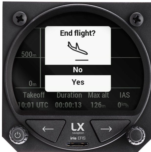
Figure 72. Manually "End flight" by pressing right-hand push-rotary knob while on Statistics page.
