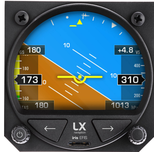
Figure 15. "Show airspeed" is enabled, "Show altitude" is enabled and "Show direction" is set to "Off"
